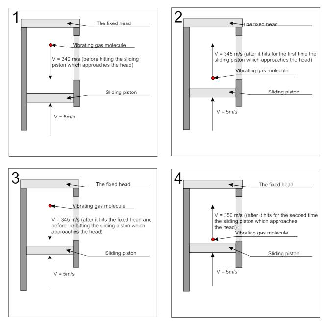
The following is an example calculation of the increase of temperatures (the speed of gas molecules vibration) for reciprocating piston engines where the following parameters were applied:
