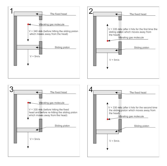
The following figures illustrate how the gas molecules behave as exemplified by a piston engine in the compression phase as the piston approaches the fixed head, vibrating gas molecules accelerate which results in heating the gas, while in the energy balance, the mechanical energy which is then transmitted from the shaft of the engine by the connecting rod on the sliding piston, is converted into the thermal energy (vibrating gas molecules).
